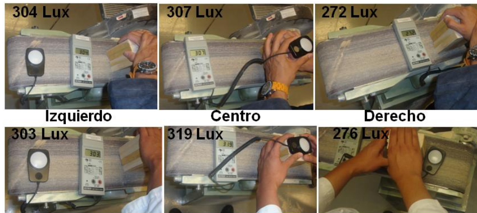
Figure 3. Lighting in new position, with dark and clear coat
